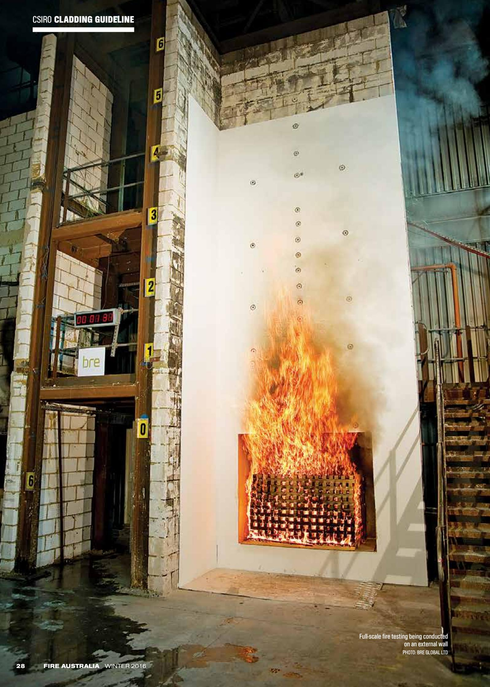
Full-scale fire testing being conducted on an external wall
