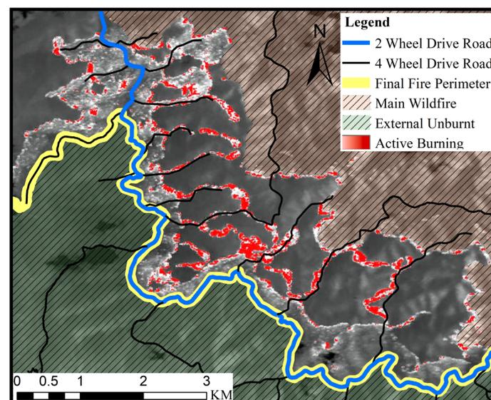
**Figure 1** Linescan image of a burnout operation in progress. The ignition pattern of this ~1,000 ha burnout uses terrain features to promote a lower intensity 'backing' fire that will burn downhill from the roads/ridgeline. A backburn has been completed along the road to secure a containment line prior to the ignition of the burnout.
