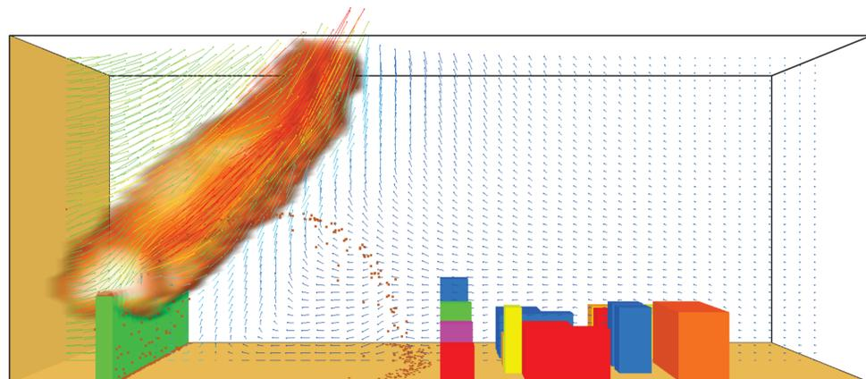
Figure2: Firebrand movement at 6 m/s wind velocity
