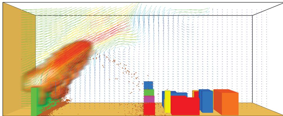
Figure1: Firebrand movement at 13 m/s wind velocity
