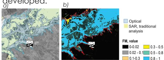
Fig 2 - a) SAR data, Surat area on Jan. 4<sup>th</sup> 2011. b) SAR-derived flood extent; FM: fuzzy membership to the flooded area. c) Performance metrics.
