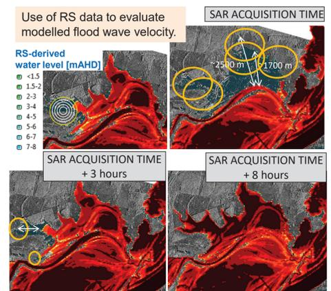
Fig 6 – RS-derived wet/dry boundary points at overpass time and modelled flood extent and depth at different times.
