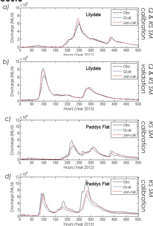
Fig 3 a) and b) Simulated catchment streamflow and c) and d) internal streamflow simulations
