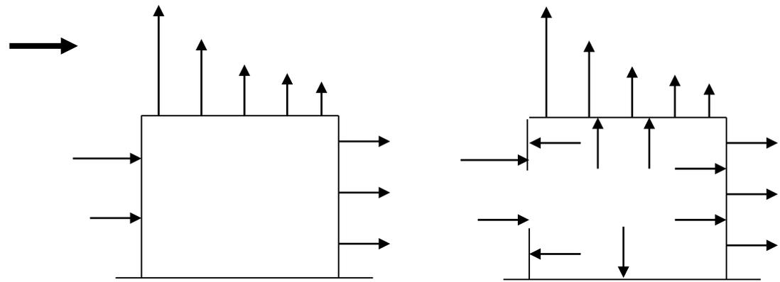
$$p, f = (0.5 \rho_{air}) [V_{des, \theta}]^2 C_{fig} C_{dyn}$$
