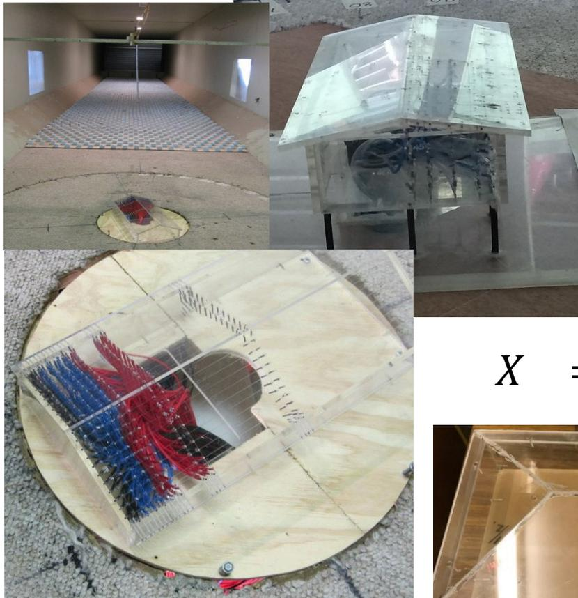
Tests in Wind Tunnel at the Cyclone Testing Station, James Cook University. On representative houses at a length scale ( $L_r$ ) of 1/50
